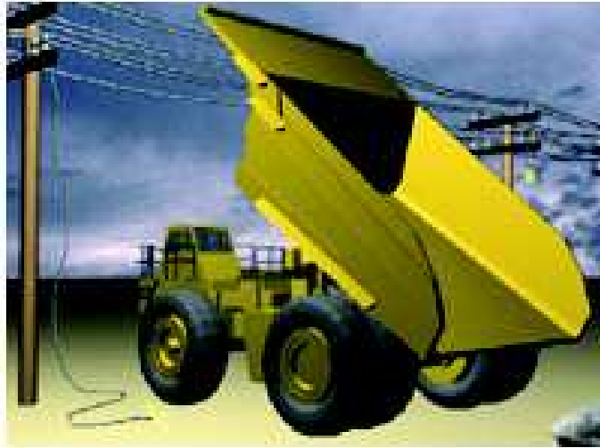
Figure 22 Dump Truck Contacting Power Lines
